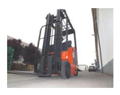
The electronic system gives to the motors the power needed to perform high travel and lifting speed, great acceleration level and unmatched maneuverability. To increase the autonomy of work several batteries of different amperage are available. The battery, removable sideways, can be replaced by using a crain or a forklift.
