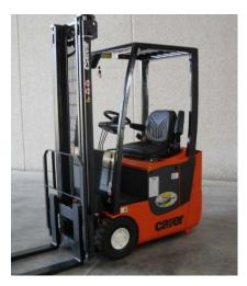
Really compact forklift width 85cm, voltage 48V, 2 ac traction motors, electric steering, rear twin superelastic tyres are some of the features that make the series N08-10 the most advanced in the industry The compact dimensions and the two front traction powerfull motors
